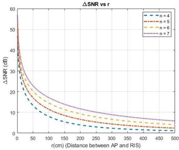
Fig. 4. Signal to noise ratio versus feeding distance
