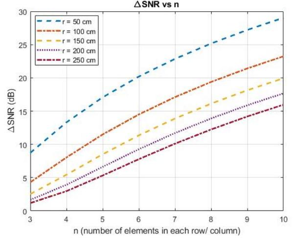
Fig. 3. Signal to noise ratio versus aperture size (element's order)
